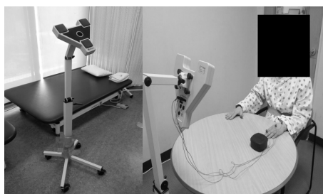
Figure 1. zebris medical GmbH CMS10(left) and figure of zebris measurement for reaching motion in study(right)
